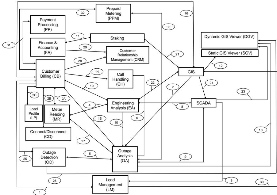
Fig. 2. The MultiSpeak software functions are shown as boxes and the defined interfaces are shown as lines connecting functions.
