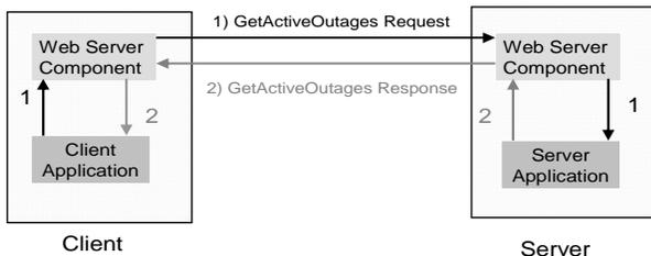
Fig. 1. Message flow to accomplish the GetActiveOutages method call. In this situation, AMR is acting as the client and OMS is acting as the server.
