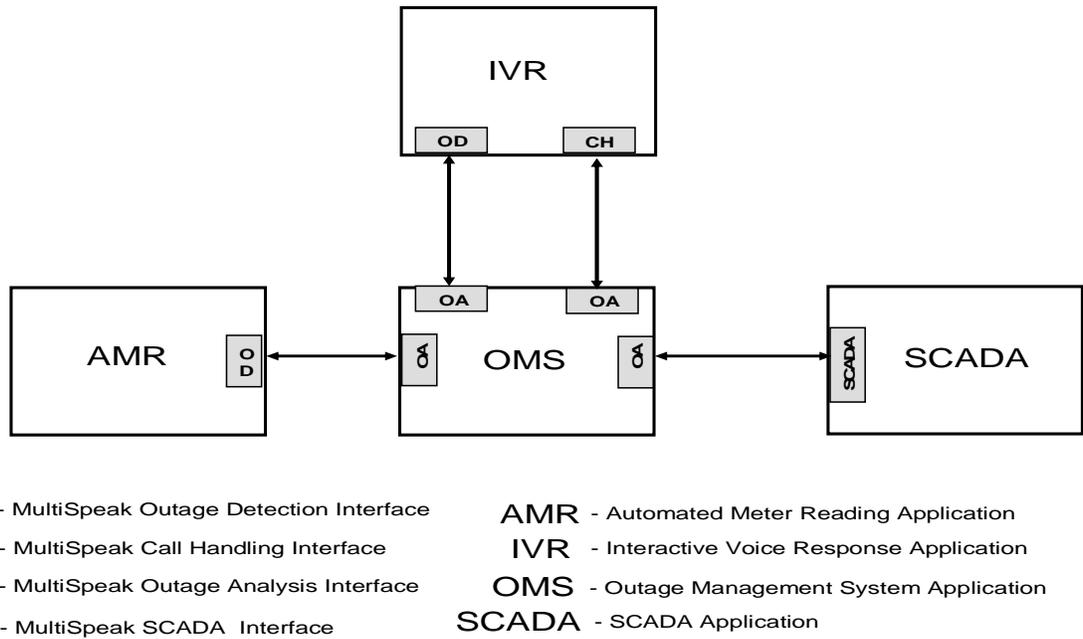
Fig. 3. This figure illustrates the software applications in place at SBEC and the relationship between those software applications and the MultiSpeak defined interfaces.
